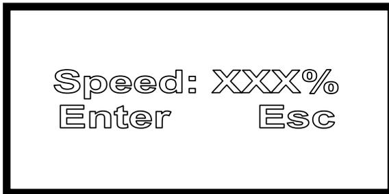
At this time press the arrow buttons to change the percentage. If you press the up and down buttons, the percentage will change at the unit of 1%; if you press the right and left buttons, it will change at the unit of 10%. After change, press the ENTER button to make the parameters function and the interface return to the system-idling one. To cancel this change, press the ESC button to return. The change of the maximum and minimum power is the same as above.
